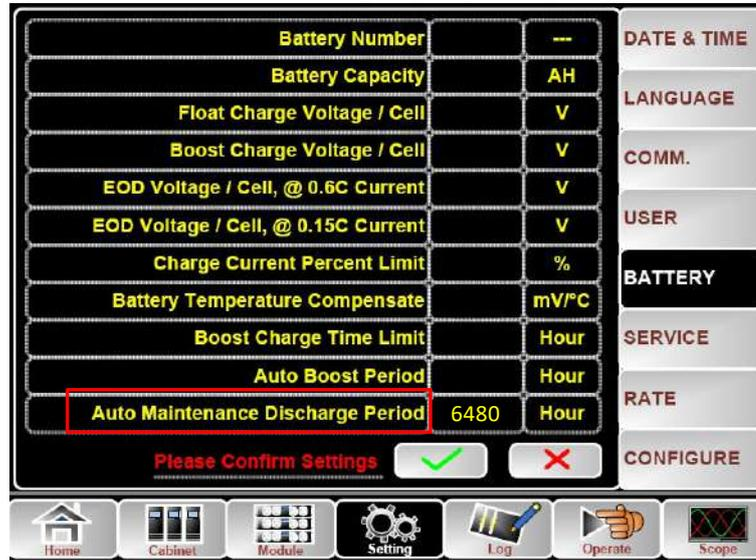
Figure 5-3 Setting period for battery auto discharge
