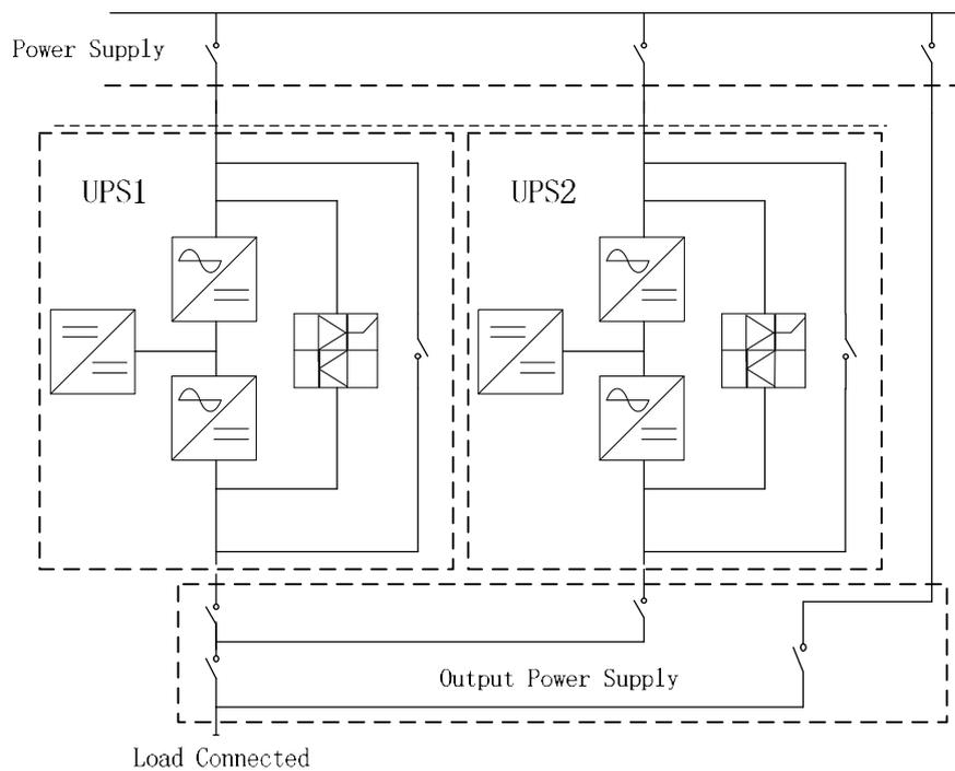
Fig. 5-6 Parallel diagram
