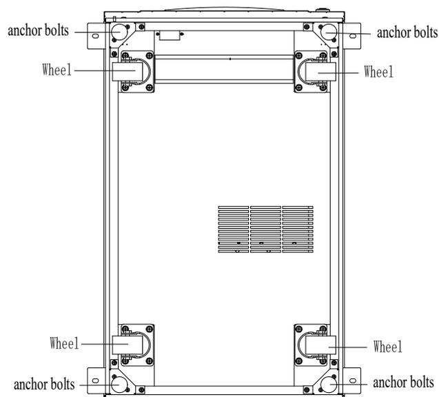
Fig.3-9 Supporting structure (Bottom view)
