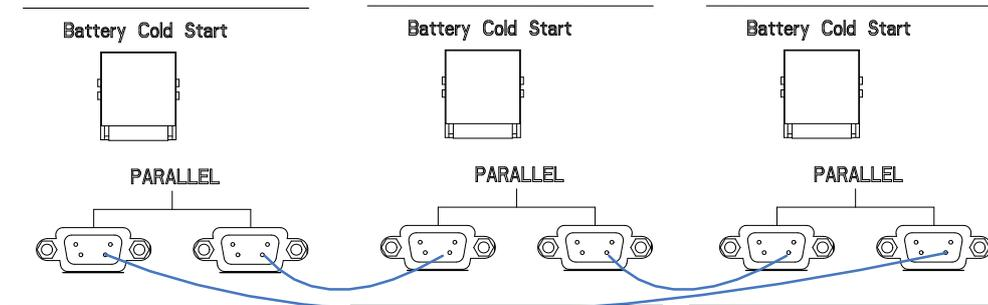
Fig.5-8 Parallel connection
