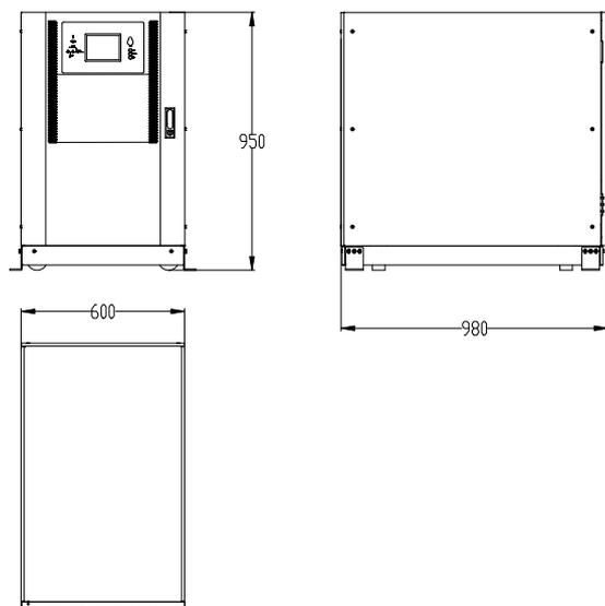
Fig.3-1 Size of the 60KVA UPS (Unit : mm)
