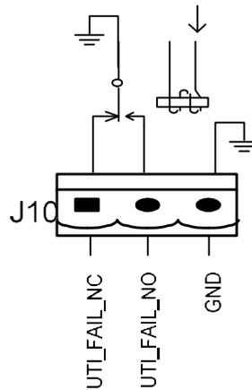
Fig.3-20 utility failure warning dry contact interface diagram
