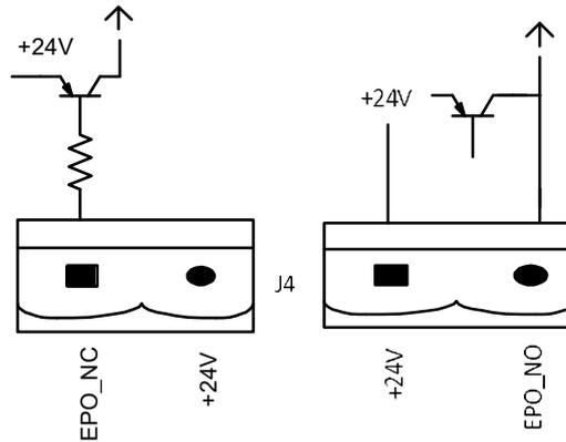
Fig.3-15 Diagram of input port for remote EPO
