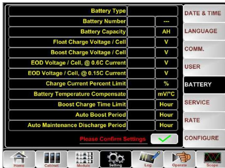
Figure 6-1 Configuration through LCD control panel
