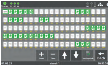
Fig. 22: Bus circuit overview - centre view
