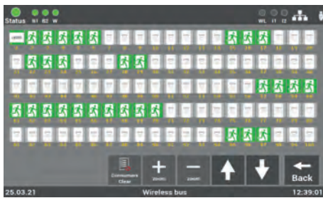
Fig. 67: "Overview Bus circuit - centre view"
